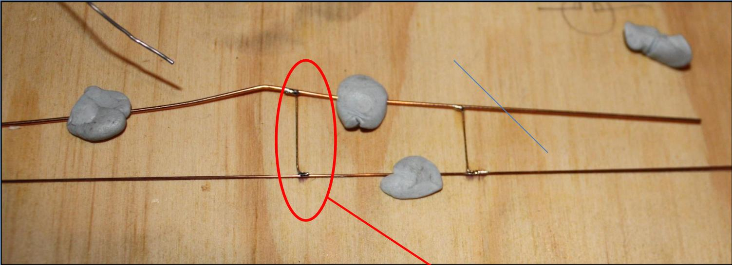
Bent droppers at angle and solder. Make sure no solder on bottom of contact wire
